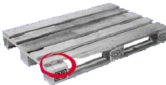
Fig.: 22: Splintered cover-wing tip edge-save
