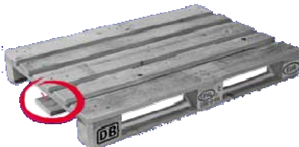
Fig.: 25: A missing block
