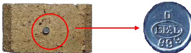
Fig.: 16 and 17: Repair marking nail
