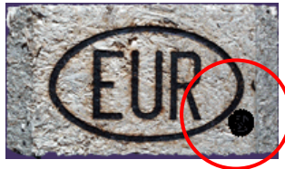
Fig.: 19: Right hitting a corner block repair marking
