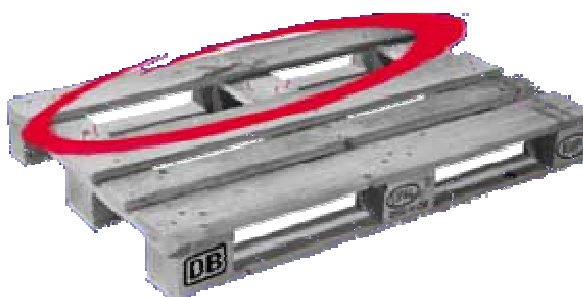
Fig.: 24: A board is missing
