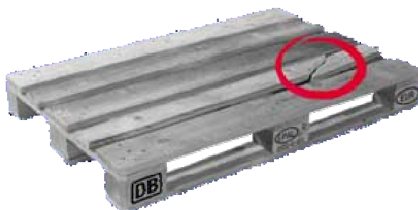
Fig.: 26: A broken board
